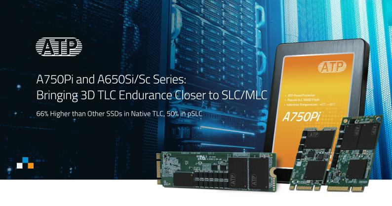
Manufactured using a new die package, the new A750Pi and A650Si/Sc Series embedded solid state drives (SSDs) are breaking endurance records. Compared with other 3D TLC drives, they deliver 66% higher endurance in native triple level cell (TLC) mode and 50% higher in pseudo single level cell (pSLC) mode, making them on par with drives built on multi-level cell (MLC) and SLC flash, respectively.
