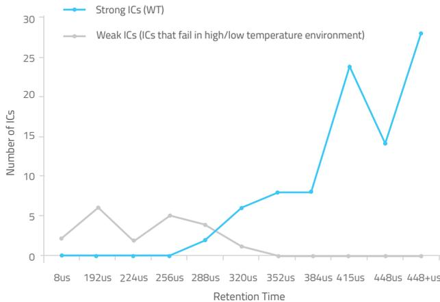
Weak ICs that fail in high-low temperature environments are screened out.
