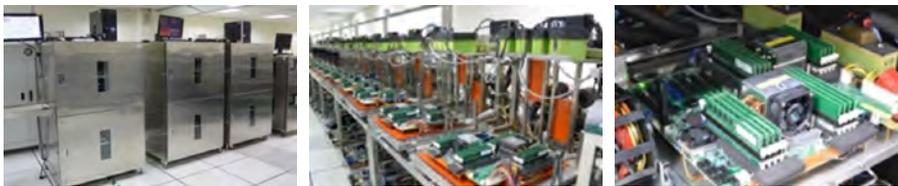
The ATP TDBI system applies extreme high/low temperature, high-low voltage, and pattern testing on DRAM modules. The system consists of:
