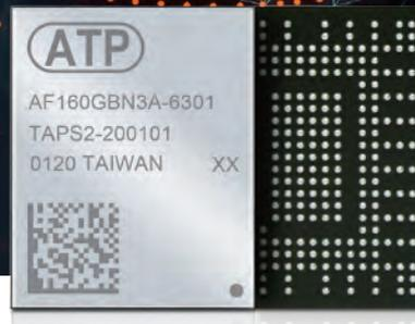
**e.MMC** offerings use a 153-ball fine pitch ball grid array (FBGA package). Smaller than a typical postage stamp, its tiny footprint makes the e.MMC perfectly suitable for embedded systems with space constraints but require rugged endurance, reliability and durability in harsh environments.
