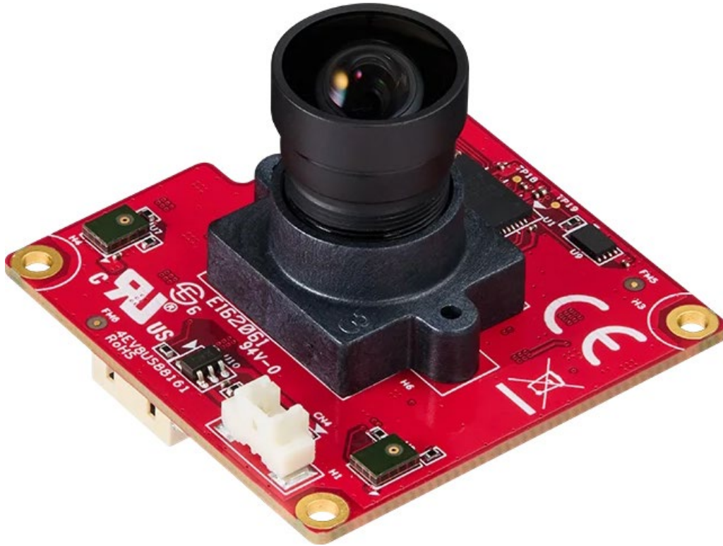
Figure 7. Above, Innodisk's EV8U-LSM-RLCF is a USB 2.0 8MP resolution, 30fps fixed focus camera module with OS support for Windows, Linux and Android. It can be used in low light conditions thanks to an integrated image signal processor (ISP) Source: https://www.innodisk.com/en/products/camera/usb-20/ev8u-lsm1-rlcf
