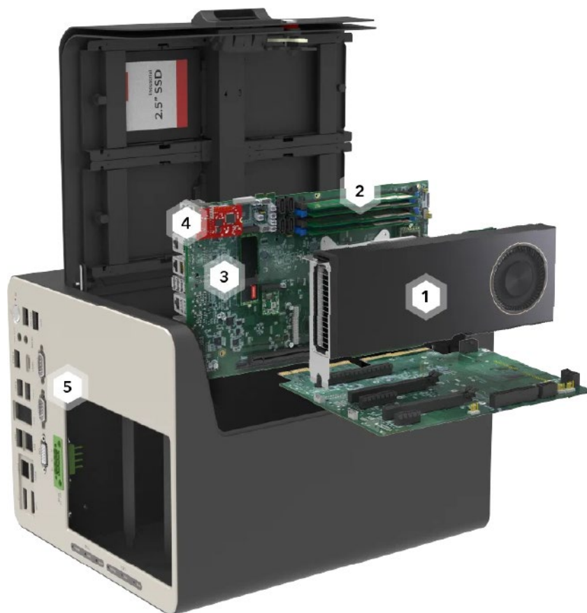
Figure 6. The APEX-X100 is an industrial / edge AI computing platform designed to support demanding vision and compute heavy workloads such as local model training, inference and fine tuning. 1 = the compute hardware. 2 = a DRAM module that supports up to four Innodisk DDR5 4400 UDIMM modules. 3 = Flash storage (featuring an Innodisk industrial-grade M.2 4TG2-P 512GB SSD with a PCIe Gen 4 x4 interface). 4 = an out-of-band remote management module. 5 = I/O ports (specifically three 2.5Gbps LANs, a 10Gbps LAN, multiple high speed USB ports and various COM/DIO ports).
