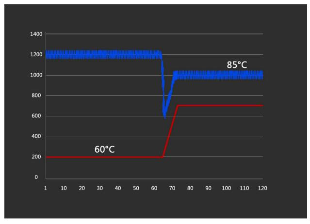
Exascend SSD with Adaptive Thermal Control. After reducing performance when the temperature reaches its threshold, the SSD gradually increases performance until it reaches a point where it can maintain stable performance at an acceptable temperature.
