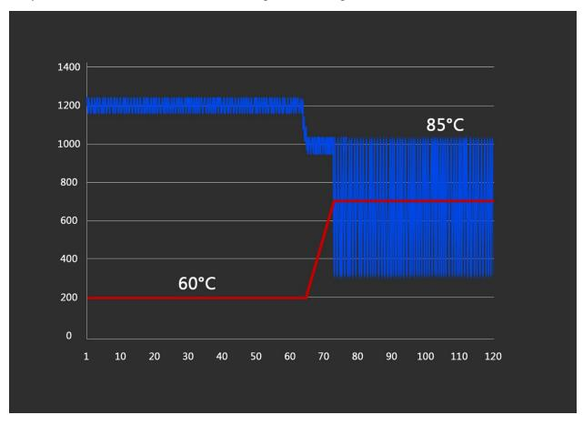
Traditional SSD with thermal throttling. The performance drops dramatically, then jumps back again when the temperature has stabilized before quickly dropping back again... and again... and again...
