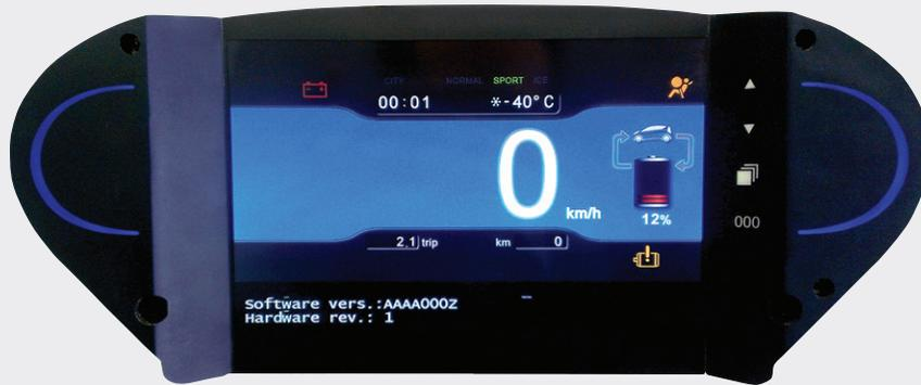
Figure 3: This electric car dashboard is driven by an Engicam SOM running Micron DRAM and NAND
