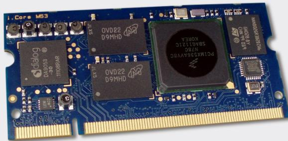
Figure 1: SOM based on the new generation of Freescale™ Vybrid™ heterogeneous dual-core processor with Micron® DDR3 and NAND
