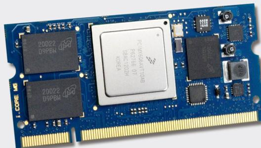
Figure 2: SOM based on the new Freescale Cortex – A9 single, dual-, or quad-core processor with Micron® DDR3 and NAND
