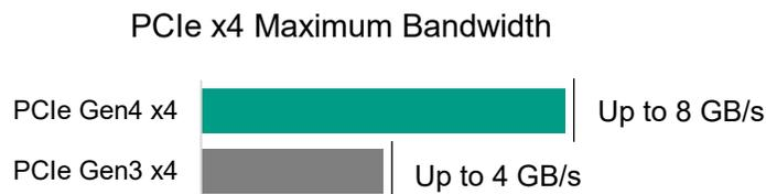
**Figure 1: PCIe Data Rate (x4 Interface Example, Maximum Interface Bandwidth)**
