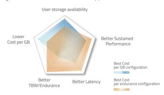
The following graph shows the new customizable pSLC-configured SATA III SSDs demonstrating significant improvements in endurance compared with default 3D TLC offerings.
