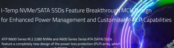
feature a completely new design of the power loss protection (PLP) array, which utilizes a new power management IC (PMIC) and new firmware-programmable MCU (microcontroller unit). The new MCU design is integrated into ATP's latest PLP technology, which allows the PLP array to perform intelligently in various temperatures, power glitches and charge states.
