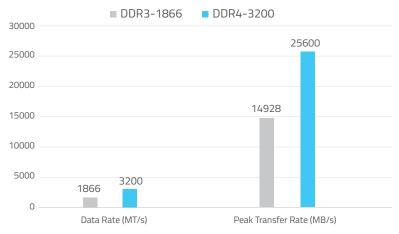
Figure 1. Performance comparison: DDR3-1866 vs. DDR4-3200
