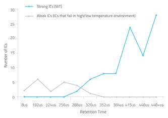
Weak ICs that fail in high-low temperature environments are screened out.
