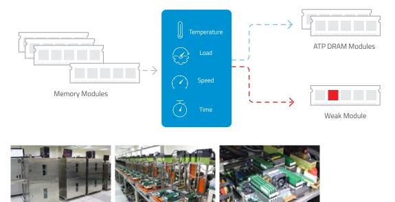
The ATP TDBI system applies extreme high/low temperature, high-low voltage, and pattern testing on DRAM modules. The system consists of:
